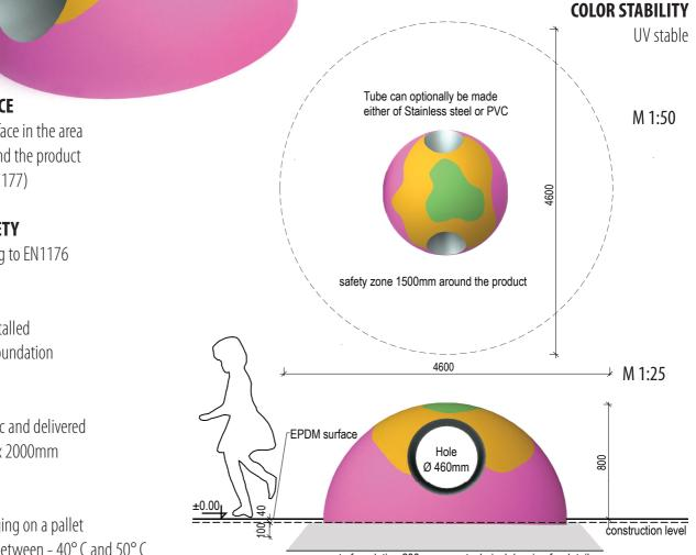
concrete foundation 200mm - see technical drawing for details
