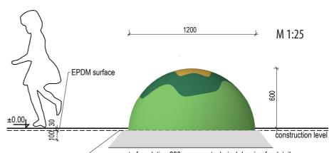
concrete foundation 200mm - see technical drawing for-details
